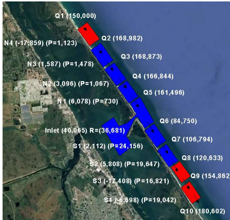
Figure 26. Annualized 14-year sediment budget for the summer 2007 to summer 2021 time period. Values on the west of the barrier island indicate sand volume changes and values on the east indicate calculated sand flux rate in cubic yards per year. P= annualized placement quantities and R = annualized value of sand removed from the sand trap. Blue cells indicate sand volume increase whereas red cells indicate sand volume loss.
