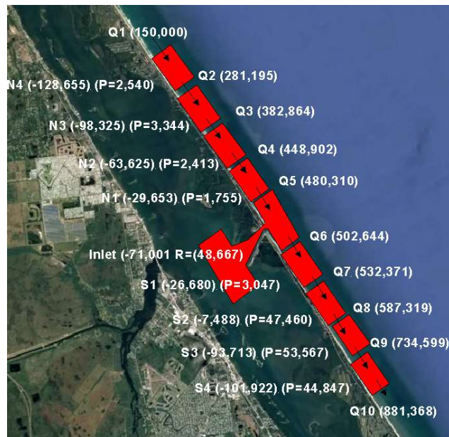
Figure 32. Annualized 3-year sediment budget for the summer 2018 to summer 2021 time period. Values on the west of the barrier island indicate sand volume changes and values on the east indicates calculated sand flux rate in cubic yards per year. P= annualized placement quantities and R = annualized value of sand removed from the sand trap.
