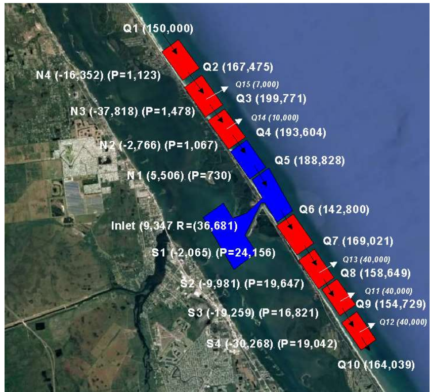
Figure 25. Annualized 14-year sediment budget for the winter 2007 to winter 2021 time period. Values on the west of the barrier island indicate sand volume changes and values on the east indicate calculated sand flux rate in cubic yards per year. P= annualized placement quantities and R = annualized value of sand removed from the sand trap. Blue cells indicate sand volume increase whereas red cells indicate sand volume loss.
