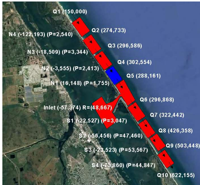
Figure 31. Annualized 3-year sediment budget for the winter 2018 to winter 2021 time period. Values on the west of the barrier island indicate sand volume changes and values on the east indicates calculated sand flux rate in cubic yards per year. P= annualized placement quantities and R = annualized value of sand removed from the sand trap.
