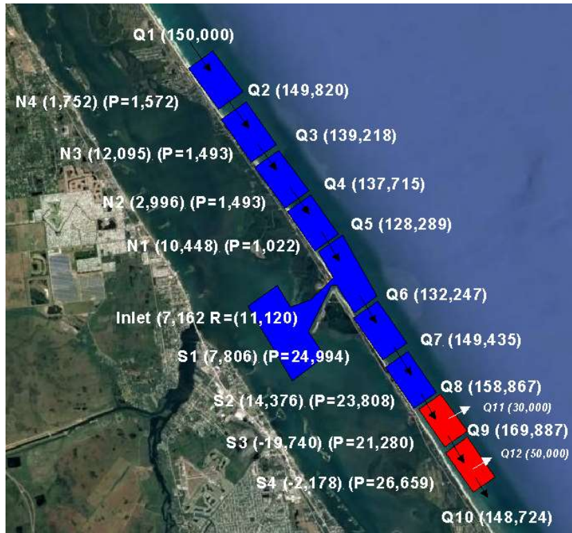
Figure 28. Annualized 10-year sediment budget for the summer 2011 to summer 2021 time period. Values on the west of the barrier island indicate sand volume changes and values on the east indicates calculated sand flux rate in cubic yards per year. P= annualized placement quantities and R = annualized value of sand removed from the sand trap. Blue cells indicate sand volume increase whereas red cells indicate sand volume loss.
