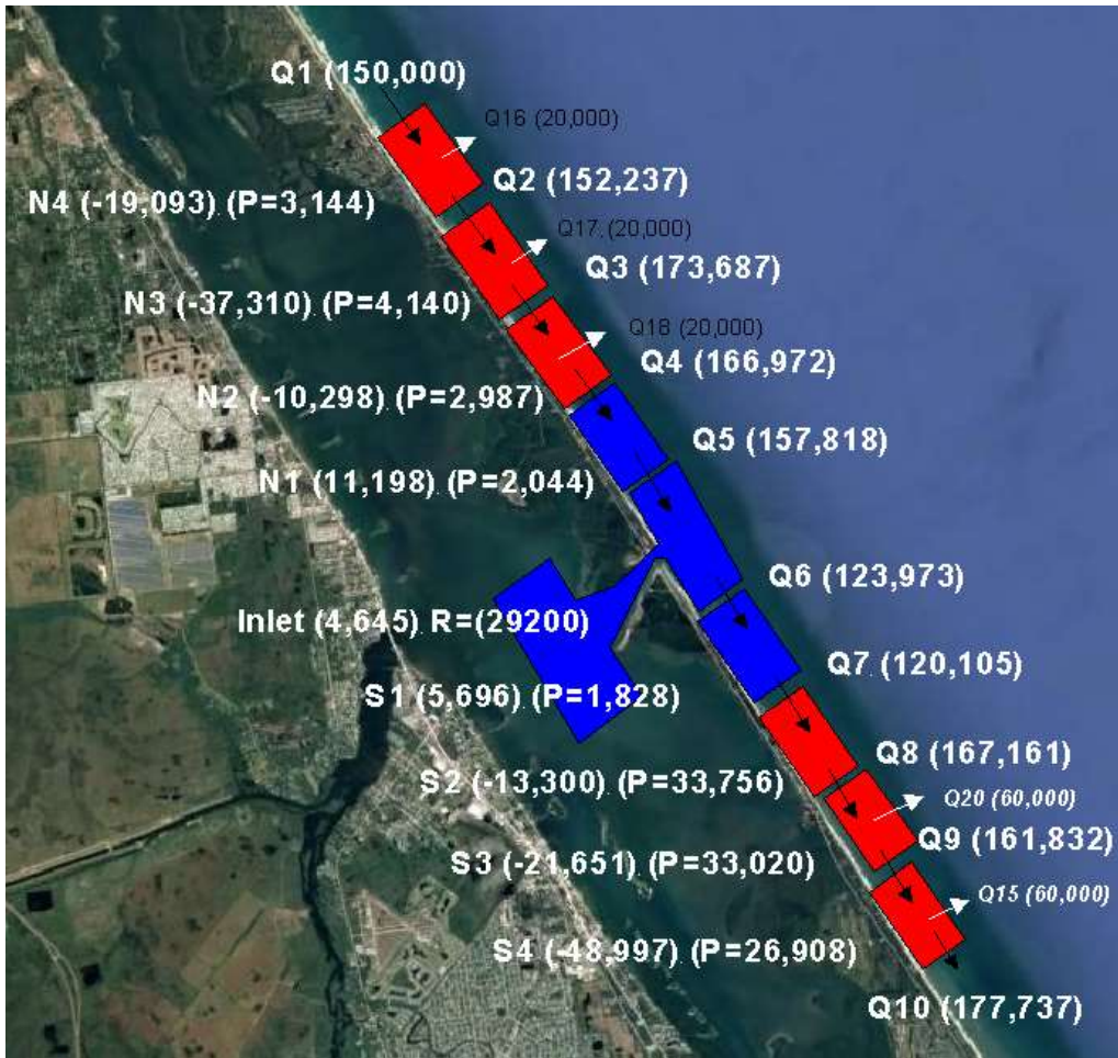
Figure 29. Annualized 5-year sediment budget for the winter 2016 to winter 2021 time period. Values shown to the west of the barrier island indicate sand volume changes and values on the east indicates calculated sand flux rate in cubic yards per year. P= annualized placement quantities and R = annualized value of sand removed from the sand trap. Blue cells indicate sand volume increase whereas red cells indicate sand volume loss.
