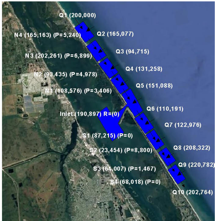
Figure 31. Annualized 3-year sediment budget for the summer 2015 to summer 2018 time period. Values on the west of the barrier island indicate sand volume changes and values on the east indicates calculated sand flux rate in cubic yards per year. P= annualized placement quantities and R = annualized value of sand removed from the sand trap. Blue cells indicate sand volume increase whereas red cells indicate sand volume loss. Onshore transport from cells N1 to N4 was required to balance the sand budget.
