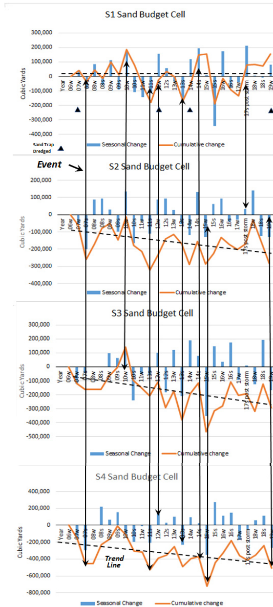
Figure 20. Comparison of sand volume changes within the Sebastian Inlet sediment budget cells S1 to S4 from 2006 to 2019.
