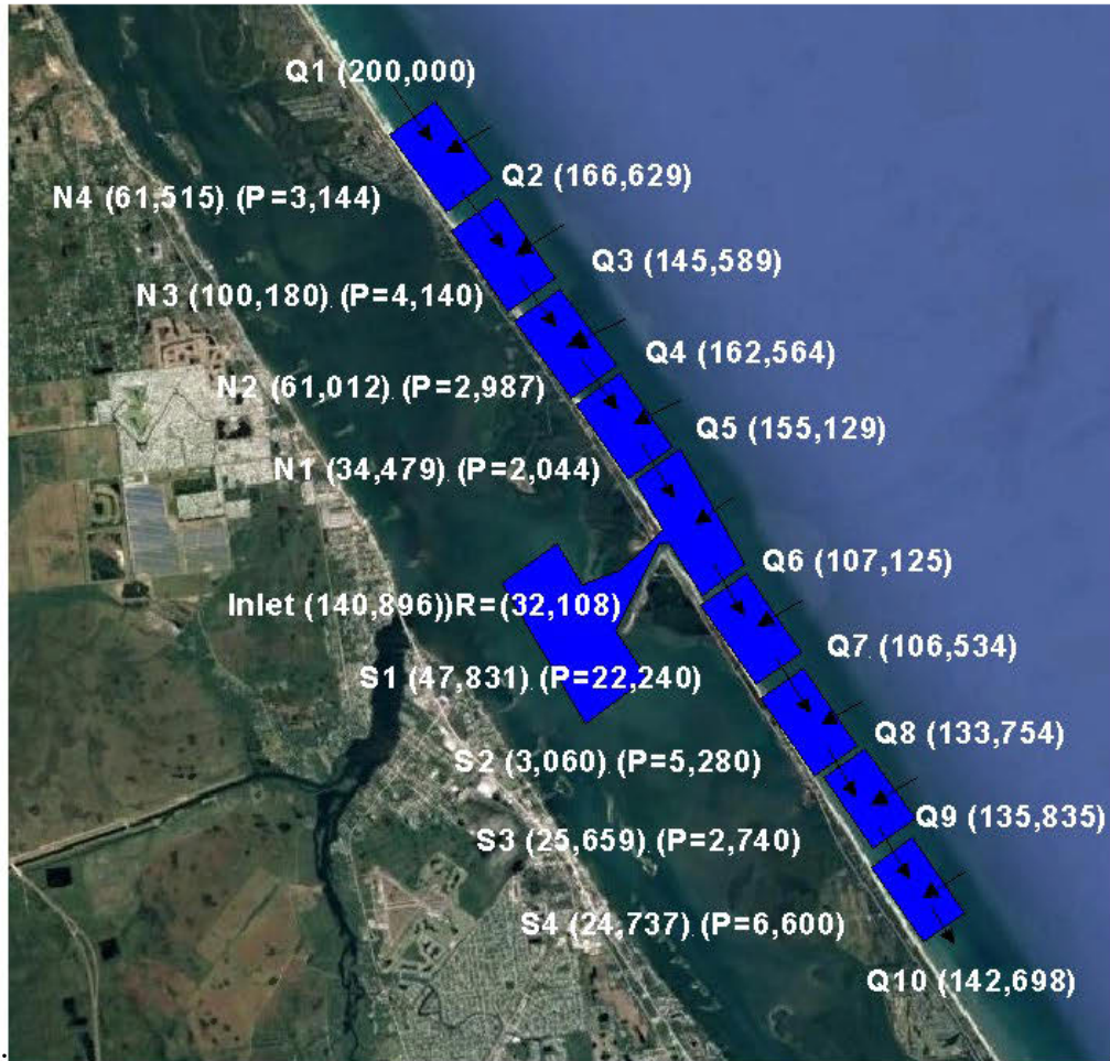
Figure 29. Annualized 5-year sediment budget for the summer 2013 to summer 2018 time period. Values on the west of the barrier island indicate sand volume changes and values on the east indicates calculated sand flux rate in cubic yards per year. P= annualized placement quantities and R = annualized value of sand removed from the sand trap. Blue cells indicate sand volume increase whereas red cells indicate sand volume loss.
