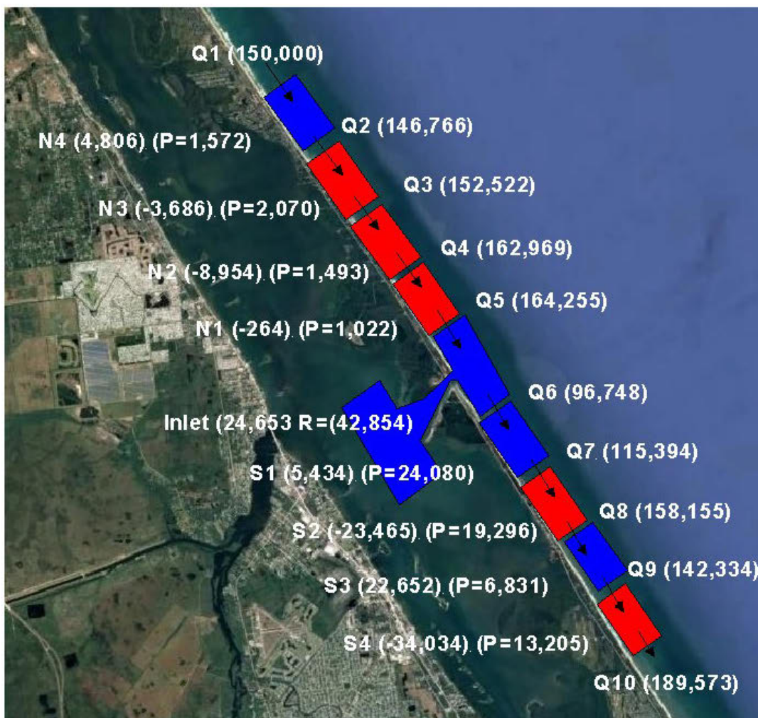
Figure 26. Annualized 10-year sediment budget for the winter 2009 to winter 2019 time period. Values on the west of the barrier island indicate sand volume changes and values on the east indicate calculated sand flux rate in cubic yards per year. P= annualized placement quantities and R = annualized value of sand removed from the sand trap. Blue cells indicate sand volume increase whereas red cells indicate sand volume loss.
