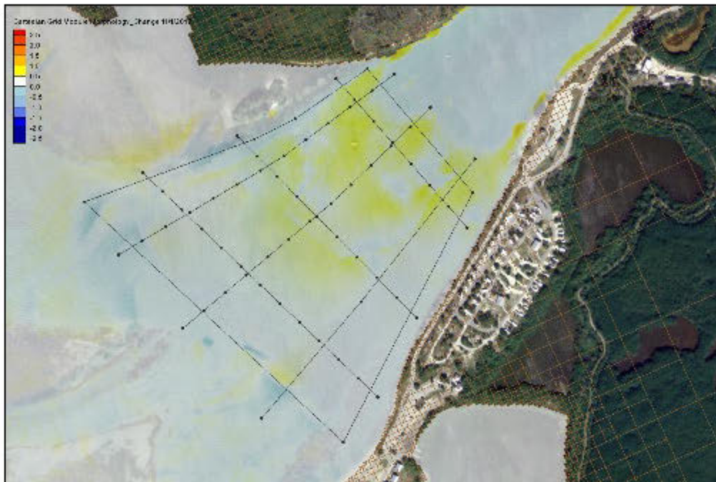
Figure 63. Calculated Morphology Change with Sand Trap Infilling Cross Sections (Post 2014 Dredge).
